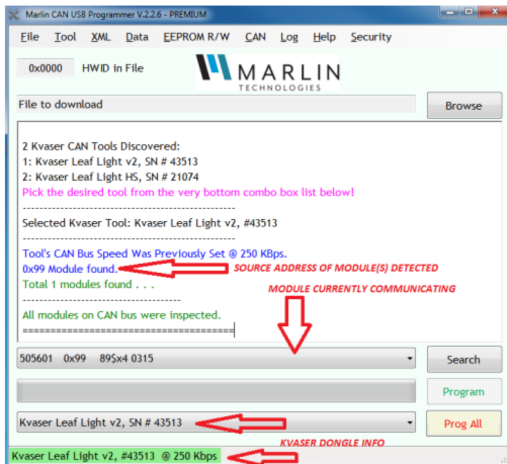
Figure 3: device being detected on the CAN bus. Shows CAN bus speed, source address and module information.
