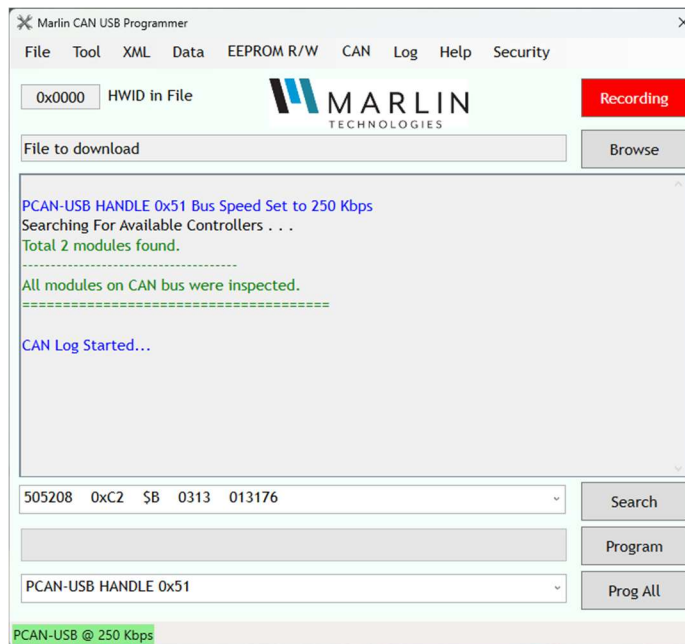
CAN logging in progress
